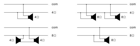
2.2 Fixed voltage (25V, 70V and 100V) output is for the convenience of connecting speaker in a long distance.
